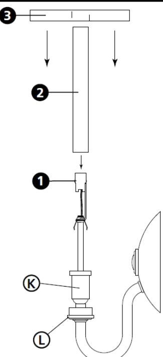
Make electrical connections from supply wire to fixture lead wires. Refer to instruction sheet (**I.S. 18**) and follow all instructions to make all necessary wiring connections. Then refer back to this sheet to continue installation of this fixture.
