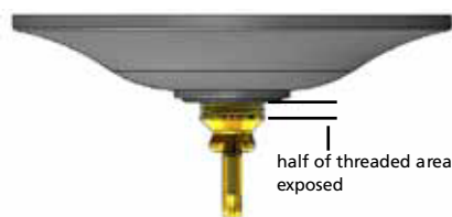
Drawing 2 Canopy Adjustment
